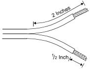
2. Strip the insulation from the ends of each conductor to expose 1/2 inch of metal wire, then twist the loose wire strands.
